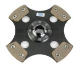
4 paddle rigid hub cerametallic drive plate. Single or twin plate format. Cerametallic drive plates have cerametallic segments riveted onto a steel back plate
